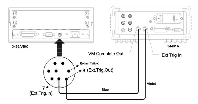
To perform a scan with the 3499 Switch and the 34401A DMM connect the two instruments as shown. You can create the cable shown by purchasing the Agilent N2289A cable, cut the DB9 connector on one end and connect BNC connectors to the Blue and Violet wire. Connect all the shields together and connect to ground. The connector that fits into the 3499A/B/C is a Miniature DIN in-line plug, 8 positions (Digi-Key PN CP-2080-ND).
